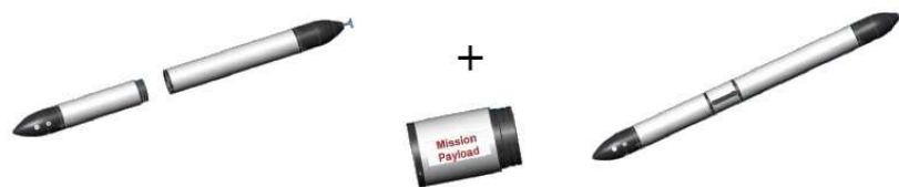
Fig.21.- AUV modular concept
